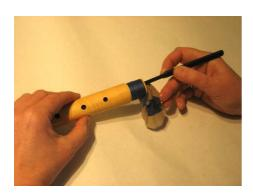
... and the middle joint, enough till the internal bore is covered by an evenly shining layer.
